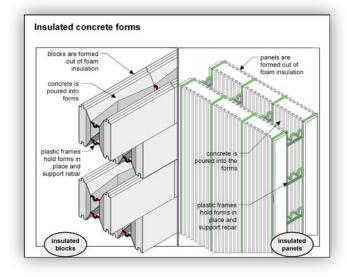
**INSULATION** ICF walls typically provide a total R-value of 22, about the same as a 2x6 stud wall. These walls also avoid thermal bridges (areas of high thermal conductivity) that are common in wood stud walls. ICF walls are also airtight, which is good for energy performance.
