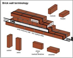
Metal ties or specially sized bricks can also be used to join the inner and outer wythes. In this case the wall will show no header courses, and it will not be apparent that it is a solid masonry wall.
