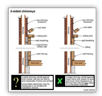
should be 12 inches of solid masonry between the wood and the flue.
