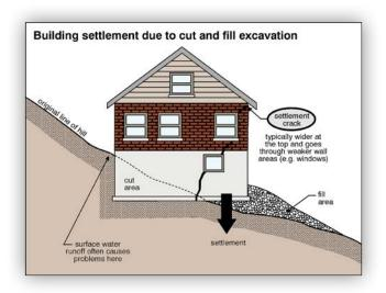
Water running down the slope is blocked by the building and accumulates here.
