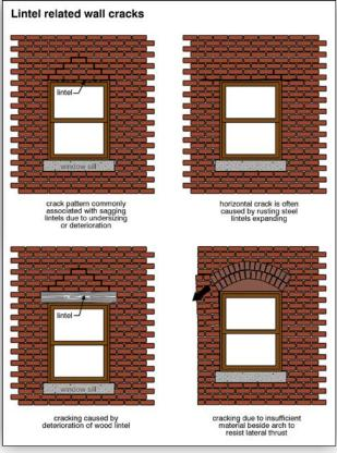
**DETERIORATION/** Mortar or masonry deterioration can, of course, lead to failure. Building settlement may allow **LEANING** the arch to open up and drop. Another problem is forward movement of the arch out away from the building. This is usually caused by foundation movement or mortar and masonry deterioration. Corrective actions include rebuilding the arch or adding a header.
