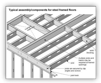
HOLES/NOTCHES Steel floor joists usually come with pre-punched holes for plumbing and electrical wiring, and should be installed so that these holes are aligned for easy installation of the mechanical and electrical systems. There are industry-specified requirements for other holes. Joists should not be notched.
