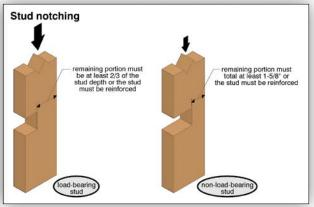
Some wood stud walls are susceptible to buckling under loads. This is particularly true if the walls are not braced with girts (blocking between studs near the mid-point) or if interior or exterior finishes are not provided. If finish is provided on one side of the wall, girts are not required.
