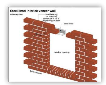
CAULKING Steel headers (lintels) supporting brick veneer should have no caulking between the steel and the brick above. Caulking may trap water and rust the steel.
