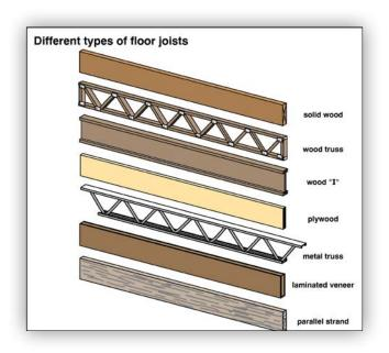
the base times the height cubed. It is interesting that two 2x10s are more resistant to bending than four 2x8s.
