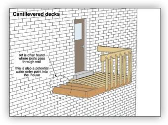
1/6 of the joist span between supports can be usually be cantilevered safely beyond a support.
