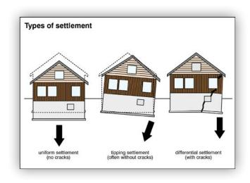
dug too deep, then backfilled to the correct depth, the disturbed soil under the footing is likely to compact over the first few years, resulting in building settlement.
