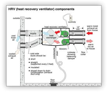
The fresh air coming into the home is filtered and then usually dumped into the return air FRESH AIR DISTRIBUTION ductwork for the furnace and mixed with the rest of the air. This distributes fresh air to all parts of the house.
