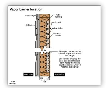
Occasionally, vapor barriers are inadvertently installed on the inside of the wall (vinyl wallpaper, for example), which can lead to water vapor being trapped in the wall and causing mold or rot.
