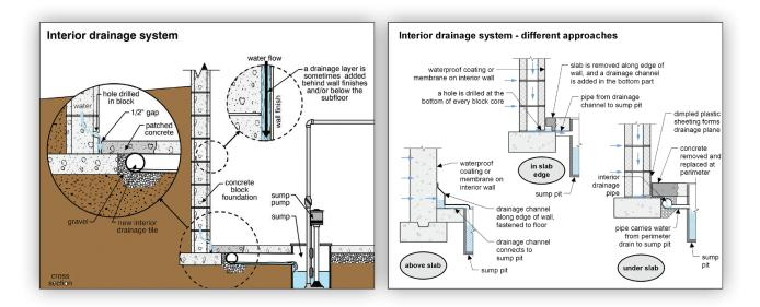
This approach is somewhat less desirable than the exterior approach, since water leaks through the exterior walls before it is carried away by this interior drainage system. The water, of course, must pass through the foundation or footing system, or go under the footing to reach this pipe. In some cases, holes are drilled through the foundation wall just above the footing to allow water to drain into this perimeter footing drain.
