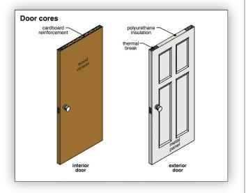
experienced when a storm door is added to an insulated metal door. The space between the doors can become overheated, and the plastic moldings may deform. In the worst cases, the metal door panel may even buckle. Many manufacturers recommend against the use of storm doors with insulated core metal doors.
