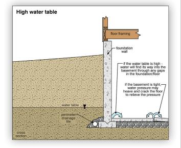
DRAINAGE Where the basement floor is below the water table, there may be chronic basement moisture problems. A drainage system and a sophisticated pumping system, sometimes with dual pumps, is often used. Since the water is constantly present, and pumps are susceptible to either mechanical or electrical failure, a house with this arrangement is always vulnerable to wet basement problems. High water alarms and battery backup systems are sometimes used.
