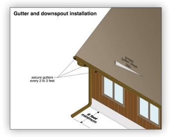
ABANDON It is common for downspouts UNDERGROUND that discharge into an under **DOWNSPOUTS** ground waste plumbing system to become obstructed or broken below grade level. This collects water outside the foundation wall, resulting in leakage. Excavating and repairing this pipe is expensive. It's much easier to cap the downspout where it goes below grade, and add an elbow and downspout extension to discharge water onto the ground several feet from the building.
