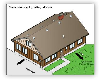
holes in foundation walls can be addressed, if needed. Large scale digging, dampproofing, drainage membranes and drainage tiles are a last resort after improving gutters and downspouts to control roof water, improving grading to drain surface water away, and correcting obvious points of water penetration.
