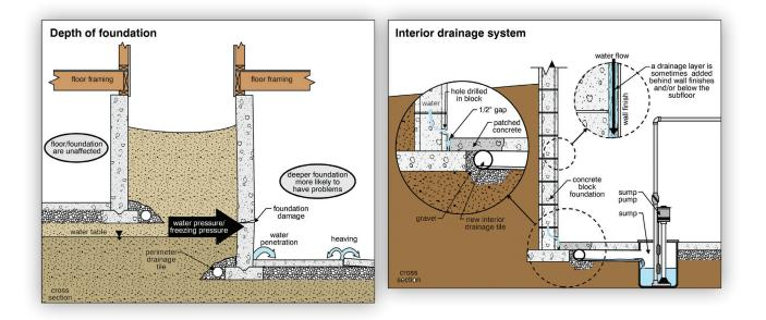
Where the water table is higher than a normal basement floor, buildings without basements are common. Slab-on-grade construction is more suitable.
