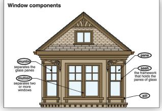
**GLAZING** Single-pane windows have a single sheet of glass. Windows with two or three panes of glass (double glazed or triple glazed) have improved energy efficiency and reduced sound transmission. These are common in colder climates. Further improvements in energy efficiency can be gained by filling the space between the glass panes with an inert gas (e.g. argon), or the addition of a low-e coating on the glass.
