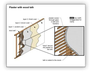
coat is called the "brown" coat and the third is a "finish or putty" coat. In a two-step process, there is still a scratch coat and a brown coat, but they are applied one immediately after the other. The finish coat is applied after the brown coat has set.
