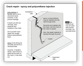
caused the crack are still present, a new crack may develop. For this reason, some contractors prefer polyurethane injection, as it stays flexible.
