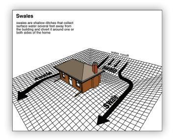
This work can be expensive where driveways, patios or sidewalks have to be lifted, although in lawn and garden areas, adding some inexpensive topsoil works fine. Sand and gravel are not effective materials, since water will flow through these easily. Well compacted soils that force most of the water to run across the surface are better.
