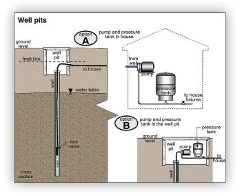
Reciprocating or piston-type lift pumps were used on older systems, while centrifugal pumps are more typical in modern installations. Shallow wells may use reciprocating or centrifugal pumps. Deep well pumps are most often centrifugal, either jet type or submersible.
