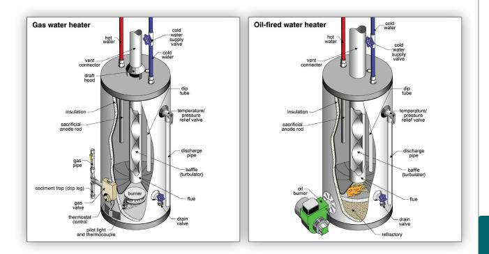
hot water, the heated water leaves the tank and cold water enters, triggering the thermostat and turning on the burner or element. If heated water flows out faster than the incoming cool water can be heated, we will run out of hot water. The larger the tank, the longer it takes to run out of hot water.
