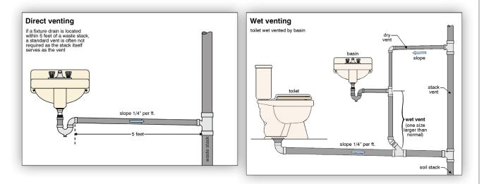
**MATERIALS** Vent piping may be cast iron, copper, galvanized steel or plastic. Because vent piping only carries air (no water) it tends to last a long time no matter what material is used.
