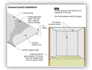
the tile and the tub is a weak spot. No matter what quality caulking is used, over a period of time, an opening will develop between the tub and tile. Although there is often a lip on the tub going up about one inch behind the tile, this does not always prevent water damage. Since bathtubs will flex to some degree, when filled with water and a person, this movement contributes to deterioration of the caulking.
