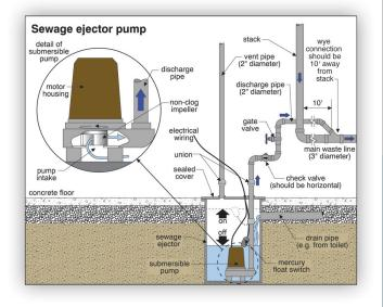
The discharge line should be equipped with a union (a connection fitting), a check valve (to prevent sewage moving backwards), and a shut-off valve, in that order.
