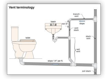
SIPHON The second function is the most important. The trap at each fixture provides a water seal
