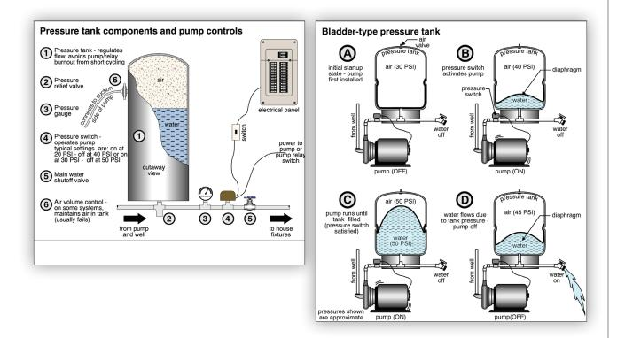
WATERLOGGED Over time, the air in the tank will be absorbed into the water and the tank will become 'waterlogged'. This means that the tank is full or nearly full of water. The pump will come on and off very quickly. This short cycling is hard on the pump, and air is added to the tank to correct the situation.
