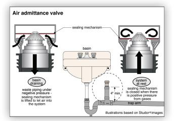
AUTOMATIC AIR While air admittance valves are approved in some areas, older VENTS style automatic air vents (see illustration), which rely on metal or rubber components, are not approved and should be replaced.
