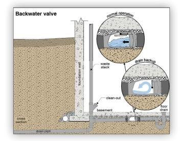
allow water down into the drain, but prevent water from coming back up. If pressures are high enough, sewage may back up through basement plumbing fixtures. In some cases, a check valve is put into the main drain line itself. These are short-term solutions and the municipality is often petitioned to improve the sewer system.
